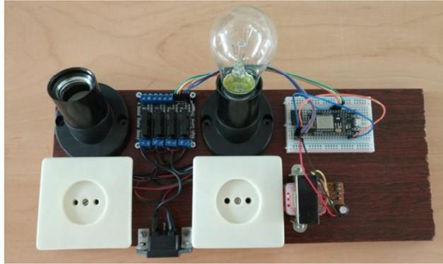
Figure 5. Ready layout project of management and control of household appliances in a smart home
