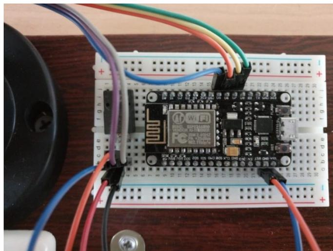
Figure 1. Board ESP8266 NodeMcu
