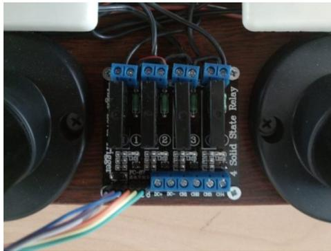
Figure 2. Relay module OMRON G3MB-202P
